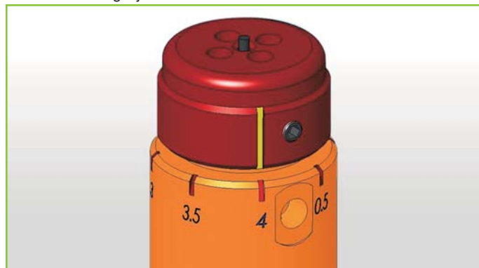
For particularly difficult applications, possibility of choking the self-cleaning piston stroke by decreasing the output section of the mixing chamber
